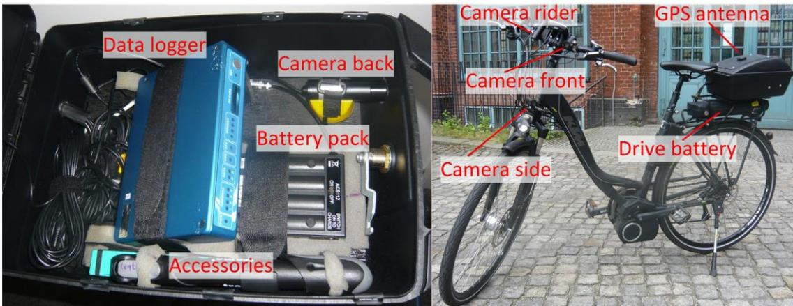
Figure 2. left: Measuring equipment on the pedelec, right: Data logger box.
